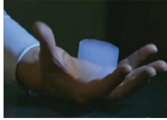
Figure 3: Aerogel ‘puffed-up sand’ or ‘frozen smoke’ [8].
