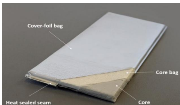
Figure 5: Vacuum insulation panel [16]
