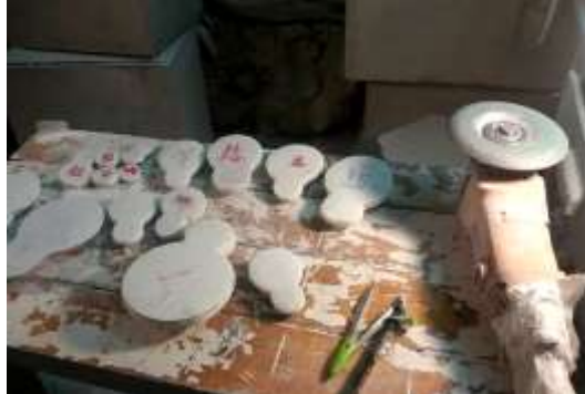
Fig.2.2 electric grinder Shaping
