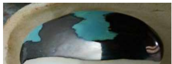
Fig.3.2 Glaze test on fired Talc (Enstatite)
